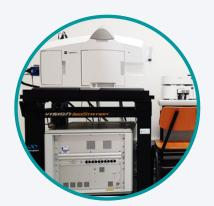
The Zeiss Lightsheet Z.1 is a lightsheet fluorescence microscope that enables fast volumetric imaging of large cleared samples (up to 1cm x 1cm x 2cm) or live transparent samples with low photobleaching and low phototoxicity.
