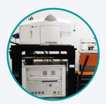
Handling, processing and visualisation of lighsheet microscopy data is extremely computer intensive and requires the use of a high performance computer. The Zeiss Lightsheet Z.1 Win 7 workstation is specifically configured for storing and handling large experimental dataset obtained with the Zeiss Lightsheet Z.1 microscope.
