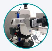
The Zeiss Axio Zoom.V16 is a motorised fluorescence stereo zoom microscope that combines a large field of zoom and working distance. It is suitable for applications in which observation and careful handling of specimens exceeds the need for greater magnification. **Applications** include microinjections, dissections, movement or separation of small organisms, and more.
