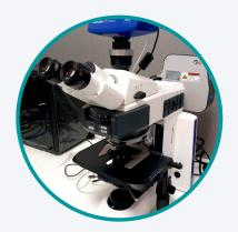
The Zeiss Axioscope 5 is a manual upright microscope with transmitted white light LED and fluorescence LED illumination Colibri 7. The Zeiss Axioscope 5 has a wide selection of objectives, including a 100x oil lens for images with increased level of detail and resolution. It is a standalone microscope, which can acquire images without the need of a computer.
