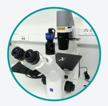
The Zeiss Primovert microscope is a manual inverted microscope equipped with the Axiocam 208 colour camera, designed for cell culture routine work.
